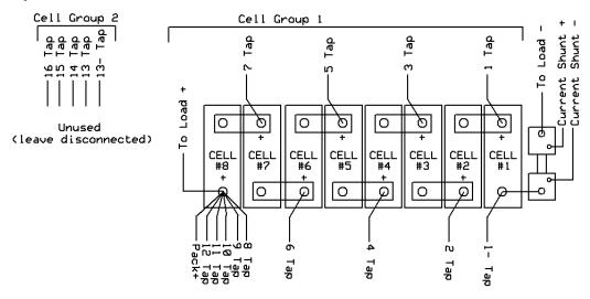
Wiring example for eight cells in series. Taps 8-12 all attach to the positive terminal on cell 8.
