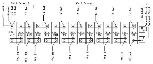
Wiring example for 15 cells in series. Tap 16 and 15 both attach to positive terminal on cell 15.
