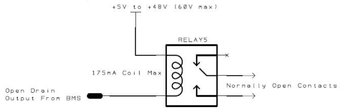
A sample schematic for connecting the open drain outputs with a relay. Note: For Rev A units, the maximum switching voltage is 24V.
