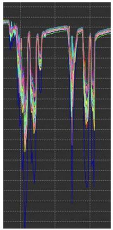
Voltage drop under load from an uncompensated high impedance busbar (blue)
