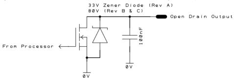
Simplified internal schematic for signal outputs
