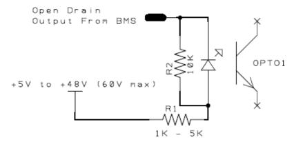
A sample schematic for connecting the open drain outputs with an opto-isolator (resistor values must be calculated based on voltage and opto-isolator requirements). Note: For Rev A units, the maximum switching voltage is 24V.
