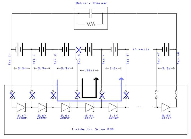
While this diagram shows a 158v battery pack, please note that the maximum voltage for the Orion Jr. BMS is 60v. However, the same principles apply.
