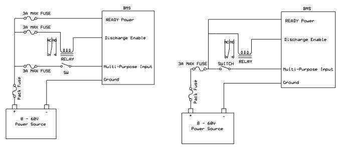
Two diagrams showing fuse placement.
