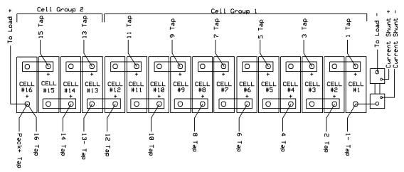
The above image is standard wiring when used with 16 cells.
