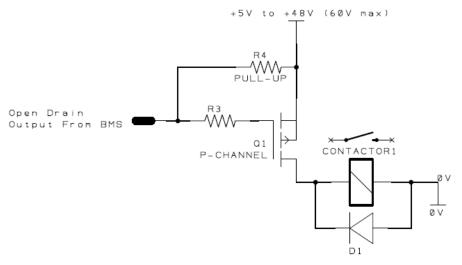
Schematic showing a P-channel MOSFET used to amplify the open drain output. Note: For Rev A units, the maximum switching voltage is 24V.
