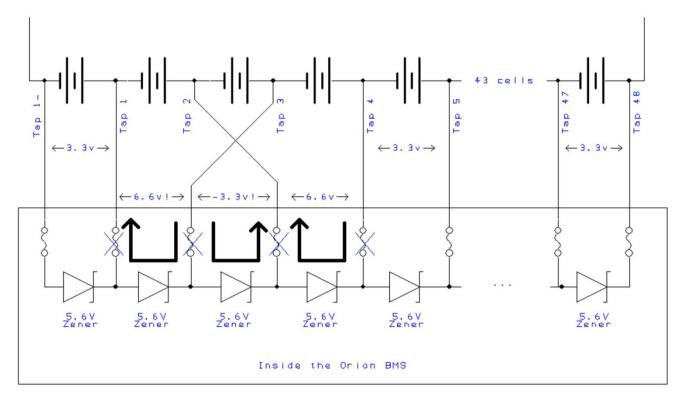
In the above schematic, cell taps 2 and 3 are reversed. This leads to 6.6v between cell taps 1 and 2 and 3 and 4 with a reverse voltage between taps 2 and 3. In this case, 4 of the zener diodes will conduct and current will flow through the tap wires. This condition leads to up to 4 fuses blown (but may be as few as 2 fuses depending on the order that they blow.) In this situation, fuses will generally reset to their normal state once the above fault is fixed.
