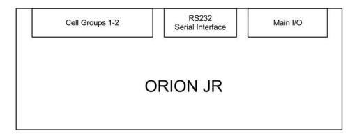
Connector locations on the Orion Jr. BMS as looking at the BMS from the top
