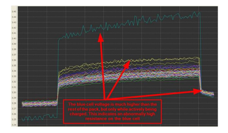
This example illustrates how an abnormally high cell resistance shows up during regular charging. Note that as soon as the charging terminates, the cell returns to a similar voltage as the rest of the pack. High resistance cells can cause pack charging to terminate prematurely because the weakest cell will hit the terminal charge voltage early.
