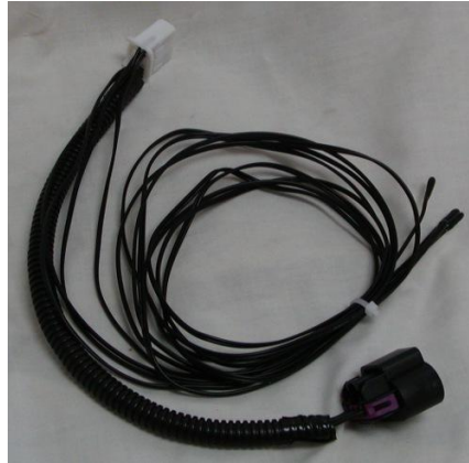
Current Sensor Harness with thermistors installed
