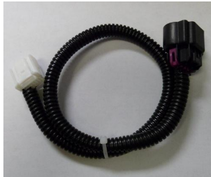
Current sensor harness without thermistors installed
