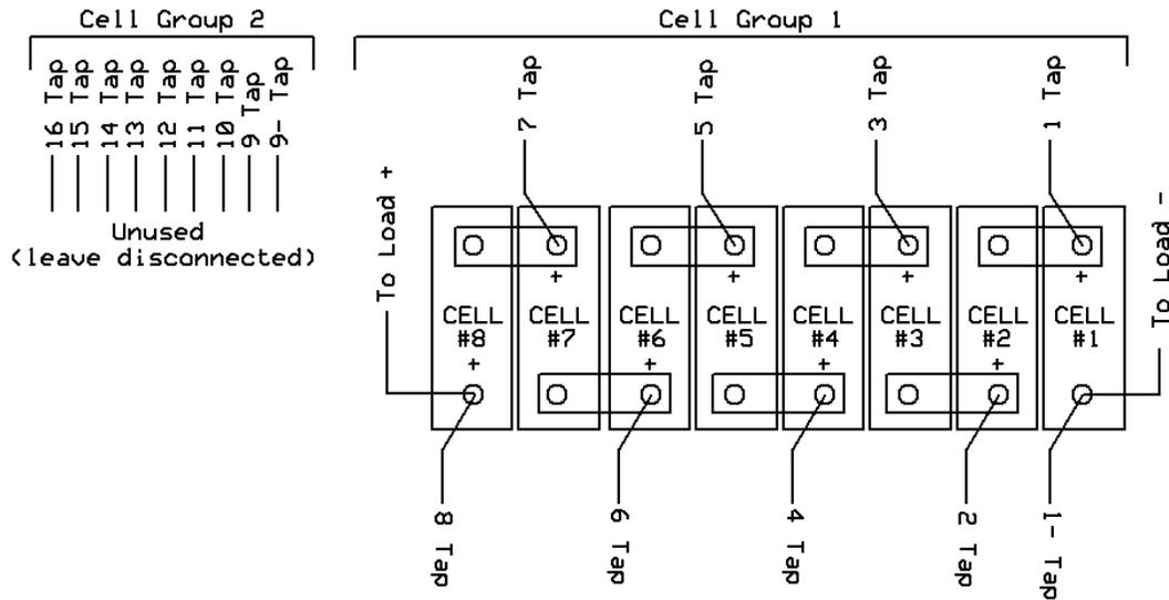
Wiring example for eight cells in series. Taps 8-16 are unused and left disconnected.
