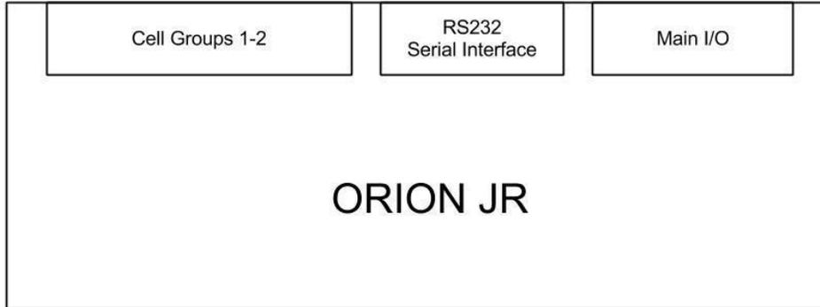
Connector locations on the Orion Jr 2. BMS as looking at the BMS from the top
