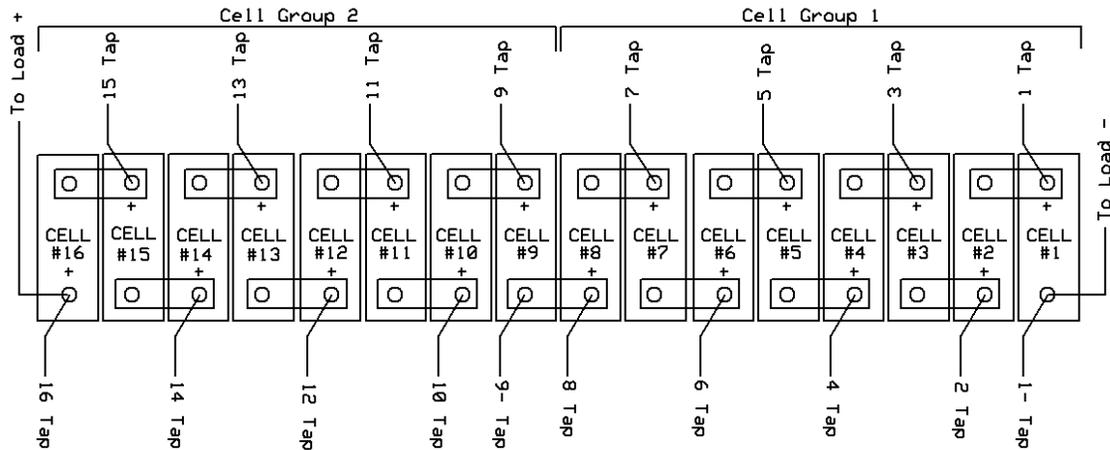
The above image is standard wiring when used with 16 cells.
