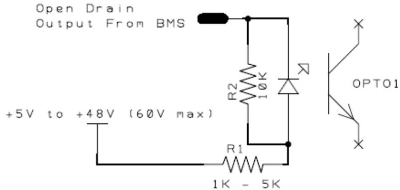
A sample schematic for connecting the open drain outputs with an opto-isolator (resistor values must be calculated based on voltage and opto-isolator requirements).
