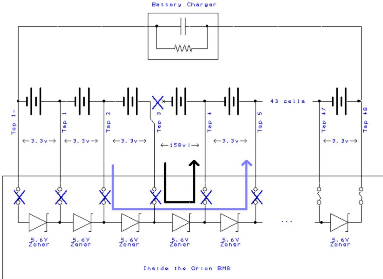
While this diagram shows a 158v battery pack, please note that the maximum voltage for the Orion Jr. 2 is 60v. However, the same principles apply.
