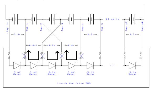
In the above schematic, cell taps 2 and 3 are reversed. This leads to 6.6v between cell taps 1 and 2 and 3 and 4 with a reverse voltage between taps 2 and 3. In this case, 4 of the zener diodes will conduct and current will flow through the tap wires. This condition leads to up to 4 fuses blown (but may be as few as 2 fuses depending on the order that they blow.) For revision E units, fuses will generally reset to their normal state once the above fault is fixed.
