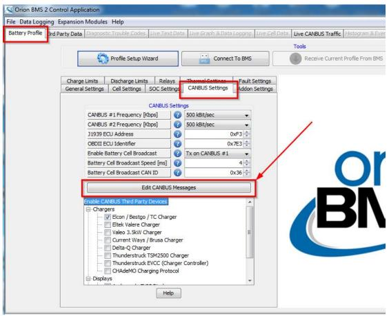
5) This dialog brings up the active (programmed) CANBUS communication matrix as shown below. This is also where the matrix can be adjusted or changed to suit the needs of the application. Selecting an individual field will display additional information (such as
