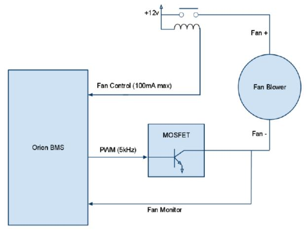
Above diagram illustrates the internal circuitry inside the BMS for the fan control
