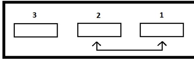
Example of swapping connectors #1 and #2 to test the wiring harness.
