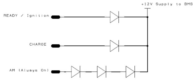
Above diagram indicates how the power supplies are handled internal to the BMS.
